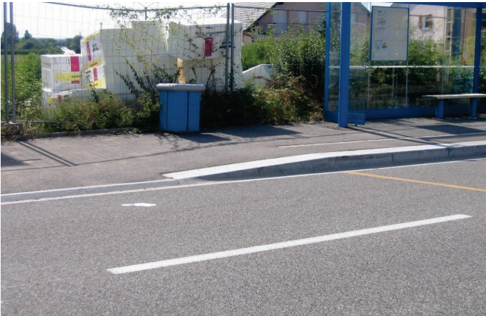
Picture of an accessible (benches, lowered portion for wheeling chairs) and secure (elevated pavement, road in good condition) pedestrian way.
